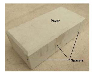
The spacers in the picture above ensure that the pavers are installed at a small distance from each other which allows sand to fill the spaces between the pavers.
